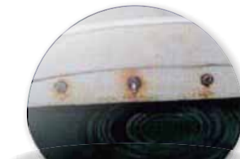
When general STS bolts are used in the air area : Corrosion occurs due to chloride gas.
