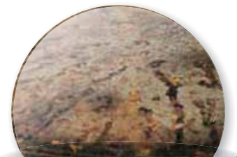
Welded type air area of the STS tank : Corrosion occurs due to chloride gas.
